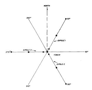
fig. 2. Sloper system using three dipoles and three reflectors with 60-degree azimuth spacing.
